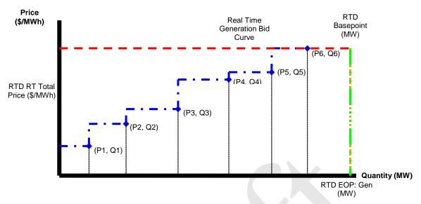
Similarly, if the RTD interval LBMP intersects the given Generation Bid block on a horizontal line and the Generator was Base Pointed within the same Bid block, the Generator's EOP is equal to its RTD Base Point.
